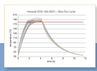
The U.S. and E.U. Pharmacopeias no longer recommend a given temperature and time for sterilization. Instead, they require proof of performance. To meet requirements of a 12 log SAL, a 6 log reduction of biological indicator endospores must be demostrated in half the time.
